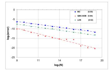
Fig. 1. RMSE versus the number of sampled points for type A model  $\sum_{i=1}^{n} (-1)^{i} \prod_{j=1}^{i} x_{j}$ . n = 360.
